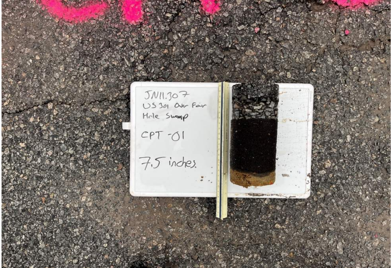
Photograph 5: Asphalt Core CPT-01
