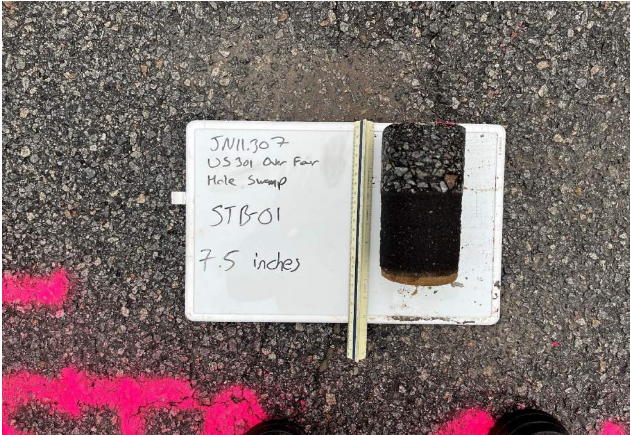
Photograph 1: Asphalt Core STB-01
